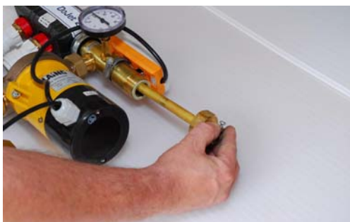
Step 4: remove entire immersion sleeve
