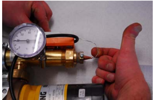
Step 13: ...with attention to soldered joint between tube and sensor (strainless fitting)
