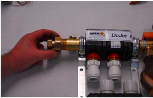
Step 8: Assemble new flange socket with seal
